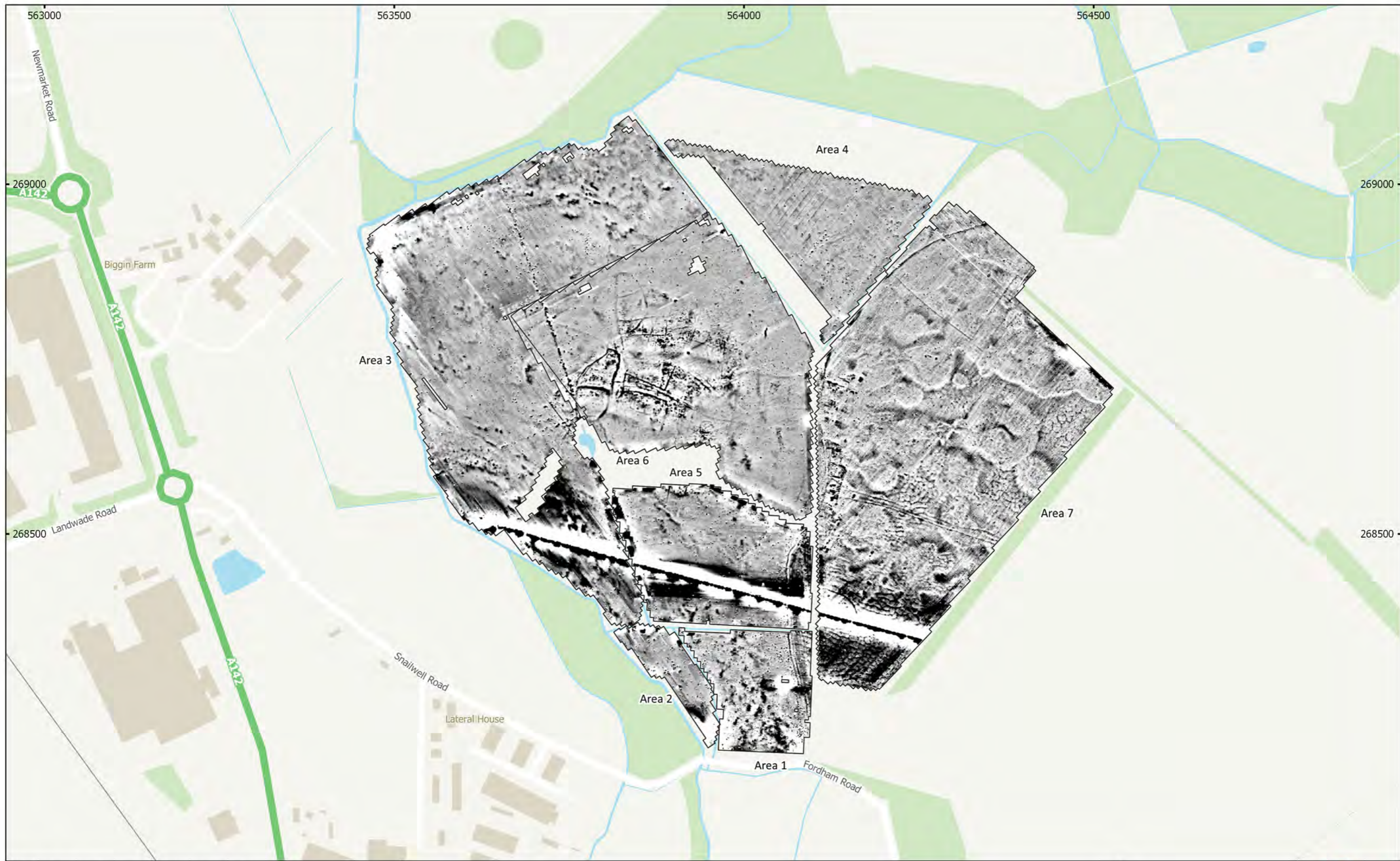
MSTL551 - Sunnica Energy Farm Reporting Zone G Figure G2 - Magnetic Total Field (Lower Sensor) (Overview) 1:5,000 @ A3 Copyright Magnitude Surveys Ltd 2020 Contains Ordnance Survey data © Crown Copyright and database right 2020
