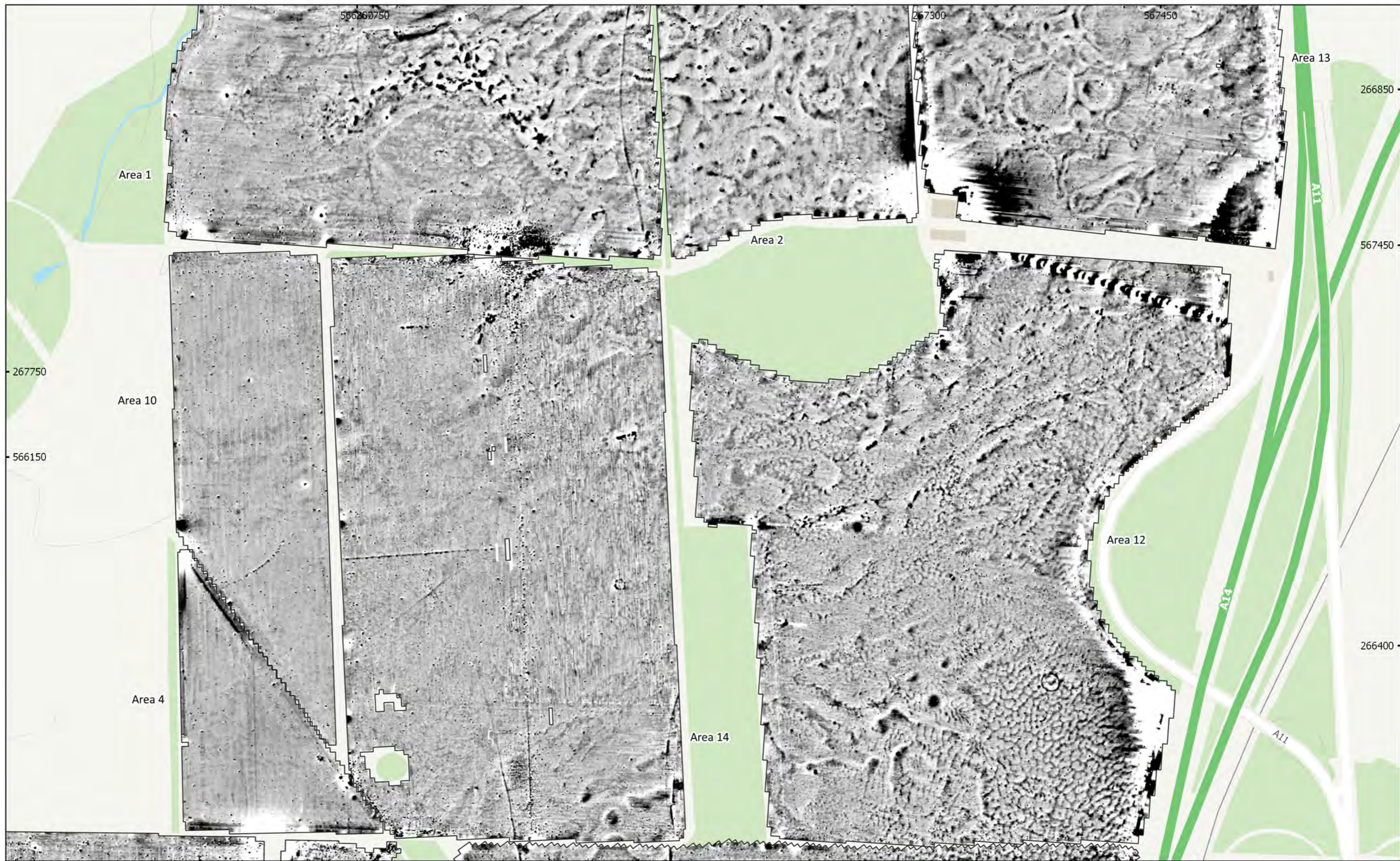
MSTL551 - Sunnica Energy Farm Reporting Zone F Figure F10 - Magnetic Total Field (Lower Sensor) (Overview) (Southeast) 1:4,000 @ A3 Copyright Magnitude Surveys Ltd 2020 Contains Ordnance Survey data © Crown Copyright and database right 2020
